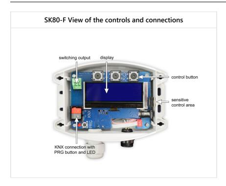
The KNX sensor is commissioned via the ETS (Tool Software) in conjunction with the associated application program. Delivery takes place in the untreated state. All functional rates are parameterized and programmed via the ETS. All parameters not relating to the KNX communication can also be set locally on the device, the lid must be loosened and open. Please note the documentation belonging to the ETS
