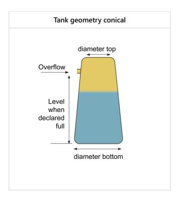
Example: lower diameter 2.5m upper diameter 1m so the ratio is 2.5, this value must then be entered.
