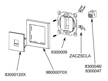
Figure 1. Single RJ45 outlet
