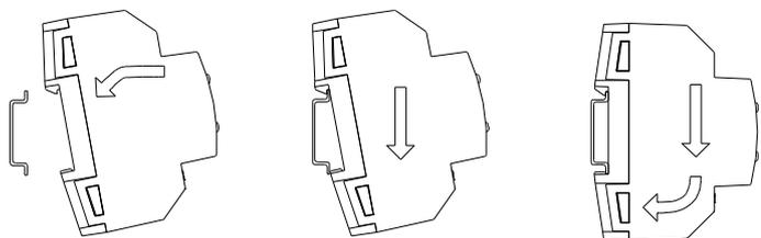
Removing DALIBOX Broadcast 6CH from DIN rail:
