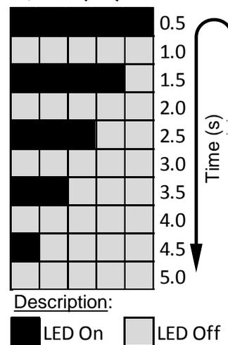
Figure 2. Error notification through DALI channel status LED
