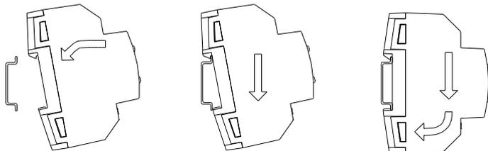
Removing HeatingBOX 230V 4X from DIN rail:
