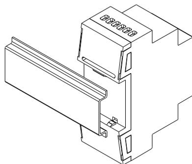
Figure 3: Mounting HeatingBOX 230V 4X on DIN rail
