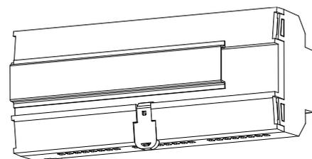
Figure 3: Mounting MAXinBOX 24 v2 on DIN rail
