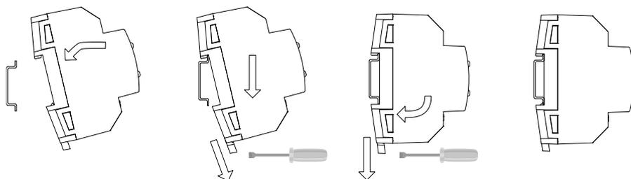
Removing MAXinBOX 24 v2 from DIN rail:
