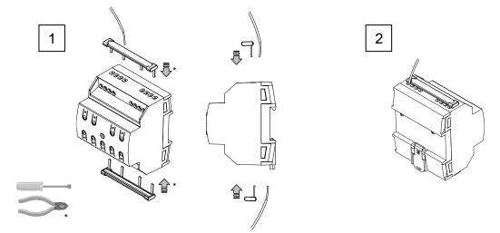
\* This accessory can be cut with a conventional cutting tool. It is recommended to remove the copper sheet to make the cut on both parts. Then, insert the cut copper sheet into the profile and cover it with another plug.
