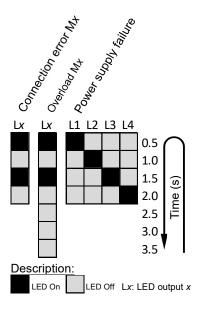
Figure 2: Error notification through grille status LED
