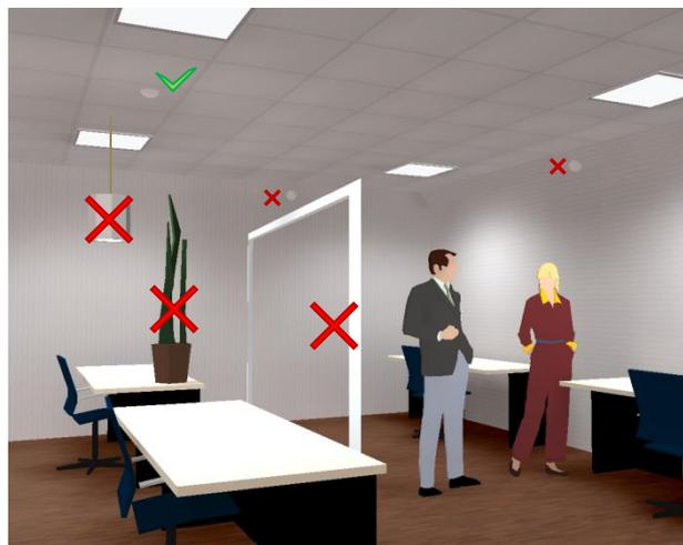
In order to improve the **Motion Detection**, it must be considered the higher sensitivity to tangential movements. Movements with axial direction to the sensor are detected worse than tangential ones.
