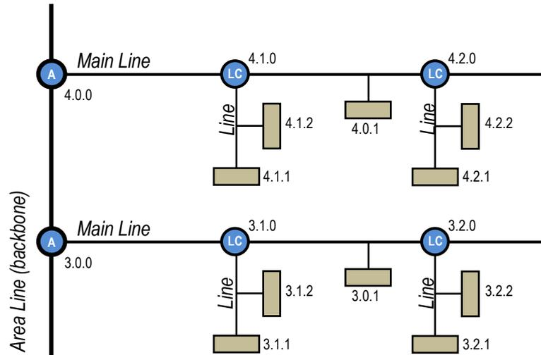
Figure 4 Line Coupling
