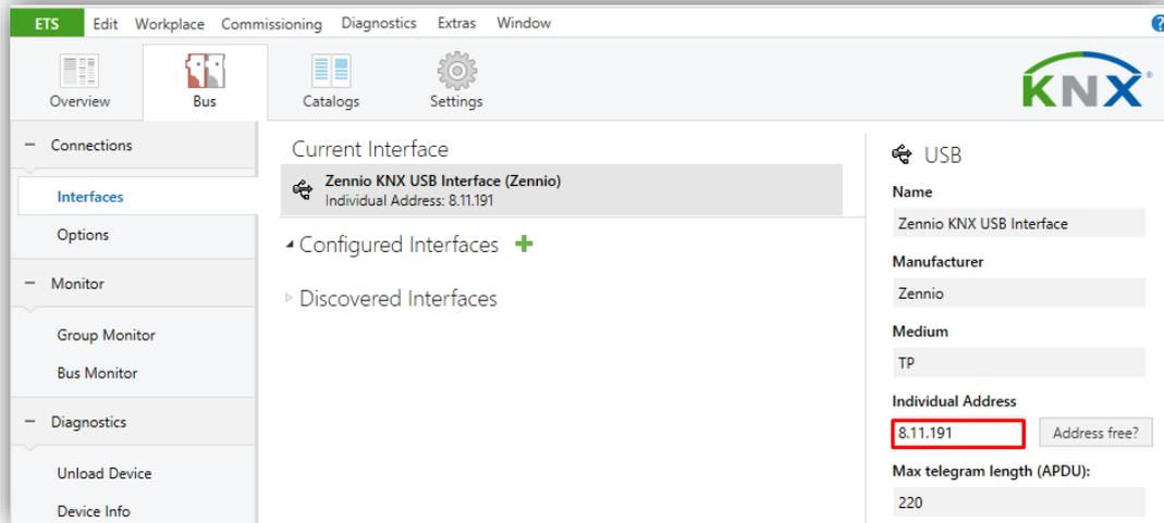
Figure 11 Configuration of the first tunneling address in ETS5.
