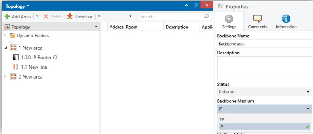
Figure 14 IP Router CL as an Area Coupler.
