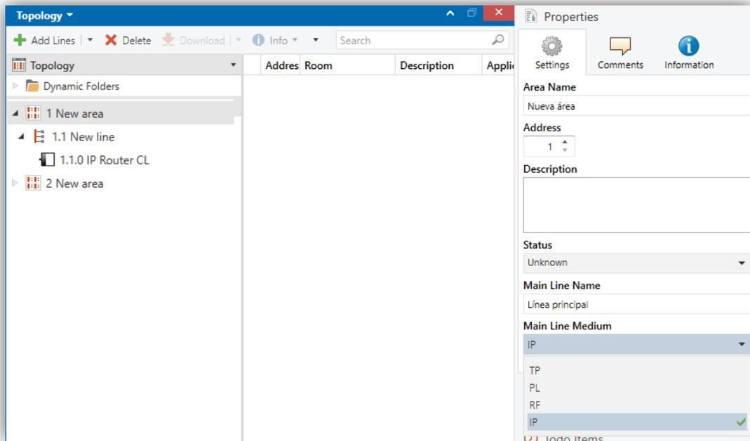
Figure 15 IP Router CL as a Line Coupler.
