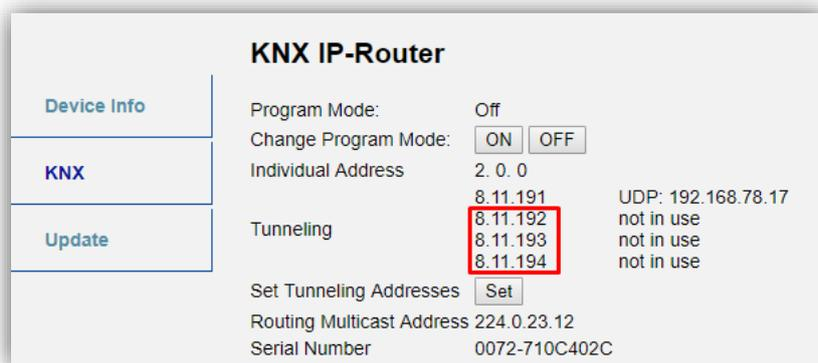
Figure 10 Set tunneling addresses in web interface.
