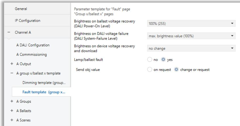
Fig 16 : Fault Template (Group x / Ballast x) Configuration
