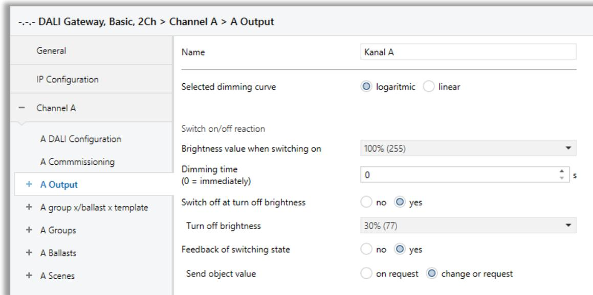
Fig 11 : A Output Configuration
