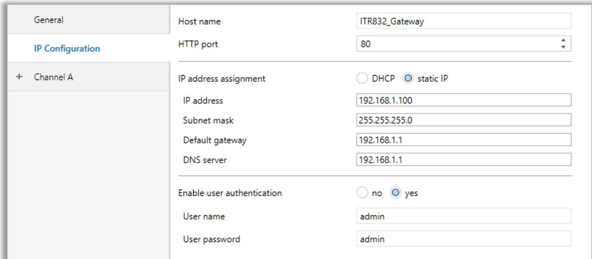
**Fig 8 : IP Configuration Parameter Page**
