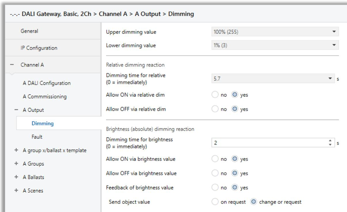
Fig 12 : Dimming Function Configuration
