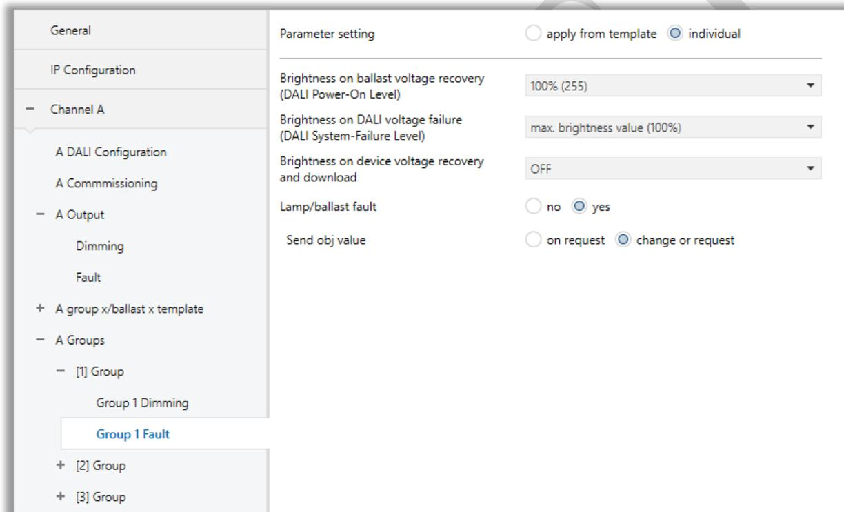
Fig 20 : Group X Fault Parameter Page Configuration
