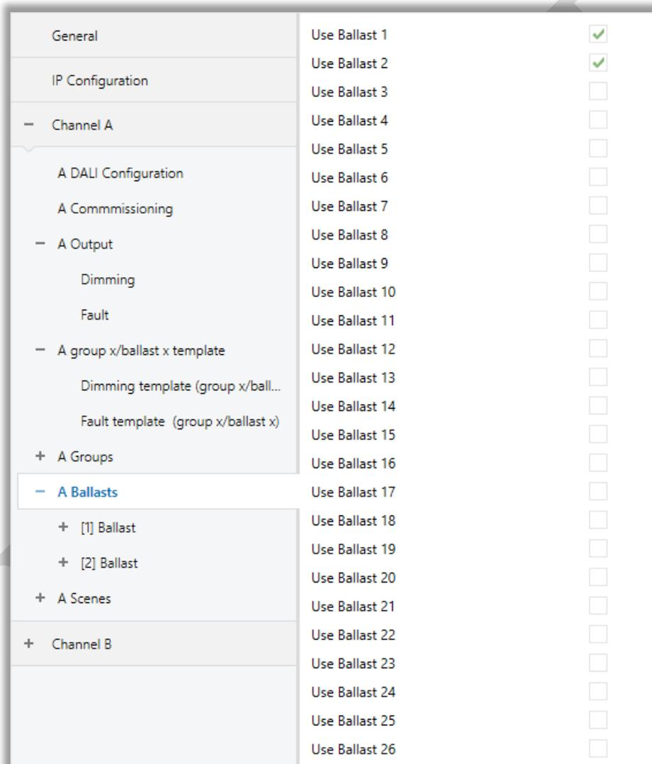
Fig 21 : A Ballasts Configuration
