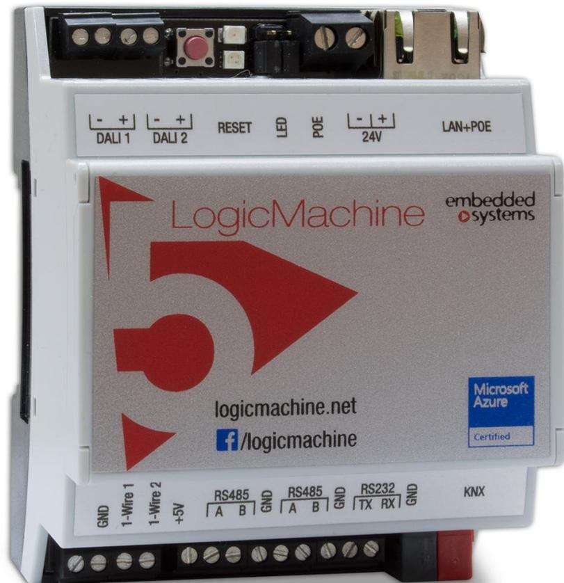
LM5 Power has Power-over-Ethernet support. Further, LM5 Power is 3x more powerful than all previous LogicMachine versions due to more powerful CPU and RAM.
