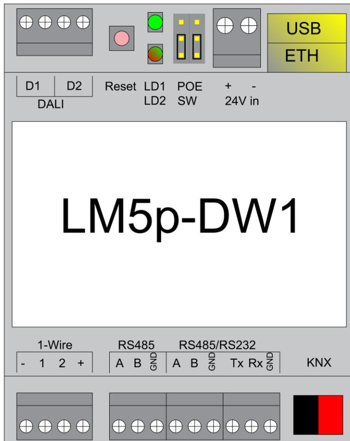
**Note!** In first batch of LM5 devices, the 24V DC clamp powering ports are placed vice versa rather than showed on diagrams!
