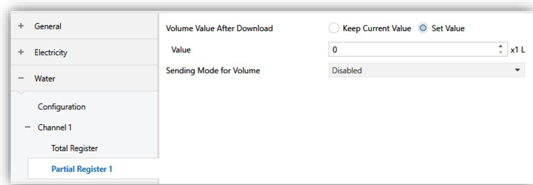
The screenshot shows a configuration window for a Partial Register. On the left is a tree view with the following items: General, Electricity, Water (expanded), Configuration, Channel 1 (expanded), Total Register, and Partial Register 1 (selected). The main area contains the following settings:
