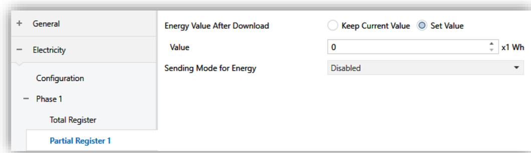
The screenshot shows a configuration window for a Partial Register. On the left is a sidebar with a tree view containing: General (expanded), Electricity (expanded), Configuration (expanded), Phase 1 (expanded), Total Register, and Partial Register 1 (selected). The main area displays the configuration for the selected register:
