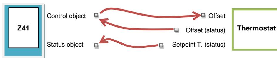
Figure 89 Relative (Float) Setpoint Control. Object Linking.
