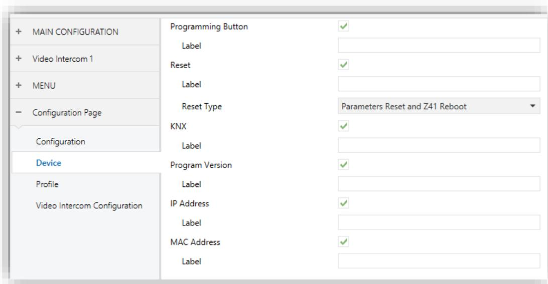
Figure 146 Device in Z41 COM (Configuration Page)
