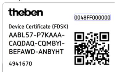
After entering the FDSK, the ETS generates a device-specific tool key. The ETS sends the tool key to the device to be configured via the bus. The transmission is encrypted and authenticated with the original and previously entered FDSK key. Neither the tool key nor the FDSK key are sent in plain text via the bus.
