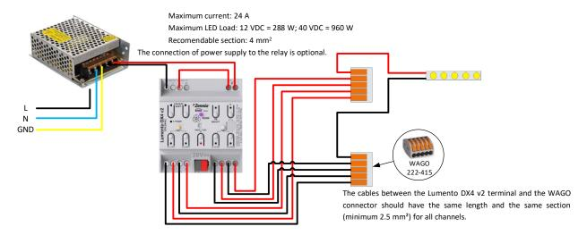
Important note: The maximum length between the WAGO connector and the LED strip should be calculated according to the allowed drop voltage for a proper regulation, the current consumed by the LED strip and the section of the cable
