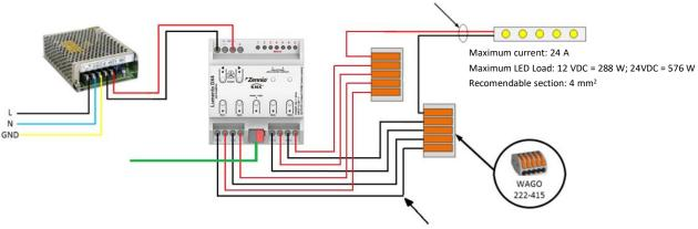
The cables between the Lumento DX4 terminal and the WAGO connector should have the same length and the same section (minimum 1.5 mm²) for all channels.
