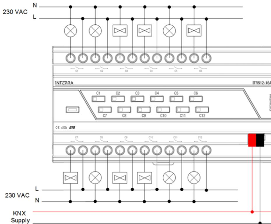
Fig21. Connection Diagram Example Configuration 1
