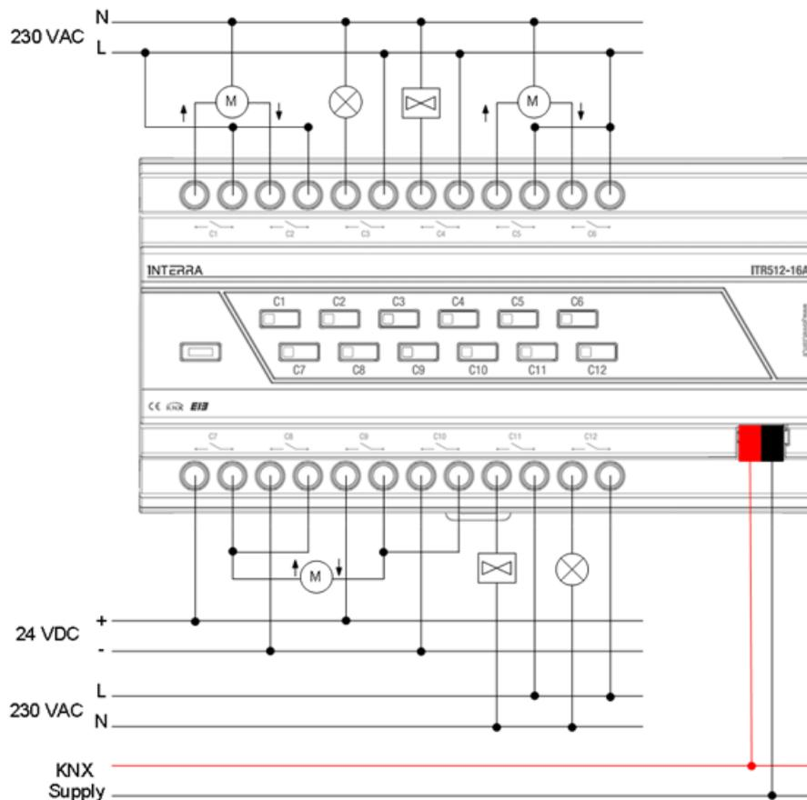
Fig23. Connection Diagram Example Configuration 3
