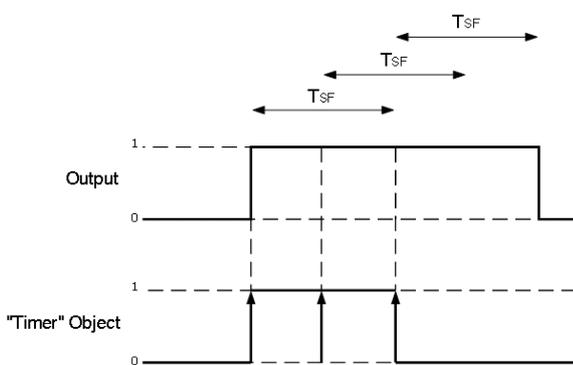
Fig3. Staircase Function Retriggerable
