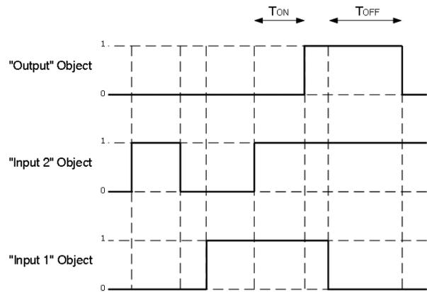
Fig1. Logic Gate with delays
