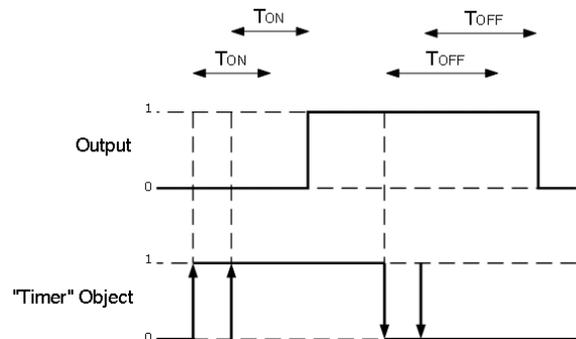
Fig5. ON/OFF Delays Retriggerable
