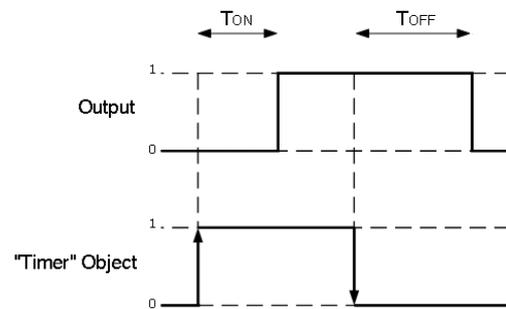
Fig4. ON/OFF Delays
