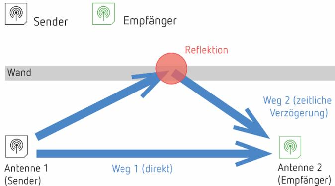
Reflections can be interference factors for radio transmission. They occur when radio signals hit obstacles and are reflected from there into a different direction. In the worst case, however, the waves received directly and via the reflection overlap unfavourably at the target location, resulting in a signal that receivers can no longer reliably evaluate.
